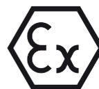
CE 0496 Ex II 2GD Ex db k c IIB T4 Ex tb IIIC T135°C IP68
